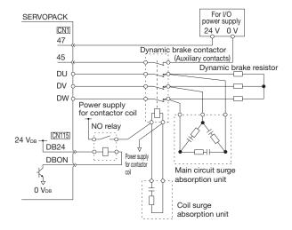
· Using NC Contacts for the Dynamic Brake Contactor
