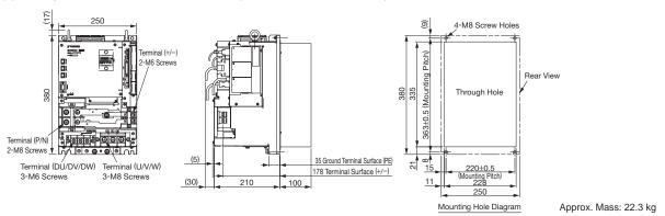
(2) Three-phase 200 VAC, 37 kW (Model: SGDV-201H)
