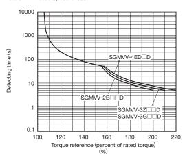
Note: Overload characteristics shown above do not guarantee continuous duty of 100% or more output.
