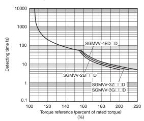
Note: Overload characteristics shown above do not guarantee continuous duty of 100% or more output. Use a servomotor with effective torque within the continuous duty zone of Torque-Motor Speed Characteristics.
