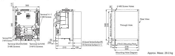
(3) Three-phase 400 VAC, 30 kW and 37 kW (Model: SGDV-750J, -101J)  $\,$
