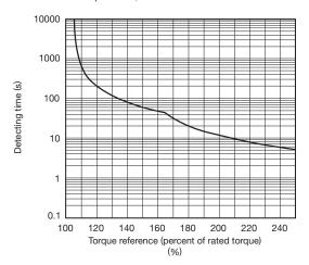
Motors with Rated Speed of 800 RPM
