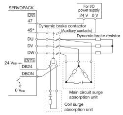
\*: The above figure is for using a dynamic brake contactor with NC contacts. The dynamic brake answer signal (a signal from NC auxiliary contacts) is input to CN1-45. To indicate an error if the input signal to CN1-45 turns OFF (open) while the dynamic brake is activated, the Pn515 parameter in the SERVOPACK must be set to n Fig. (default setting).
