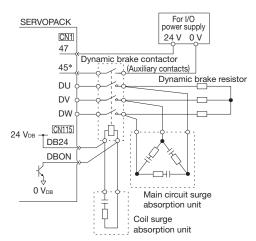
\*: The above figure is for using a dynamic brake contactor with NO contacts. The dynamic brake answer signal (a signal from NO auxiliary contacts) is input to CN1-45. To indicate an error if the input signal to CN1-45 turns OFF (open) while the dynamic brake is activated, the Pn515 parameter in the SERVOPACK must be set to n. E . If the dynamic brake answer signal is not used, Pn515 is set to n. Oderall setting).
