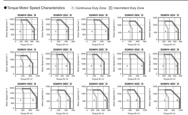
Notes: 1 When the effective torque is within the rated torque, the servomotor can be used within the intermittent duty zone.
