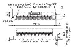
• External Dimensions of Cable (Units: mm)
