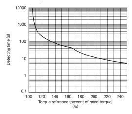
Motors with Rated Speed of 800 RPM
