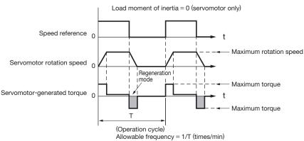
Use the following equation to calculate the allowable frequency for regeneration mode operation
