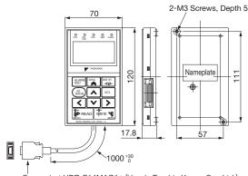
Connector: HDR-E14MAG1+ (Honda Tsushin Kogyo Co., Ltd.) Case: HDR-E14LPA5 (Honda Tsushin Kogyo Co., Ltd.)
