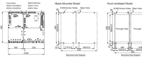
(2) Three-phase 200 VAC, 30 kW (37-kW converter and 30-kW SERVOPACK) Three-phase 400 VAC, 37 kW (55-kW converter and 37-kW SERVOPACK)
