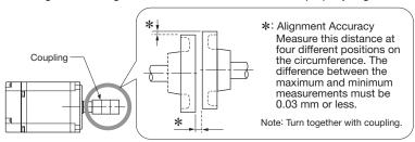
2 Do not allow any direct impact to the shafts when installing the couplings. Do not hit the area near encoders with a hammer etc., as impacts may damage the encoders.
