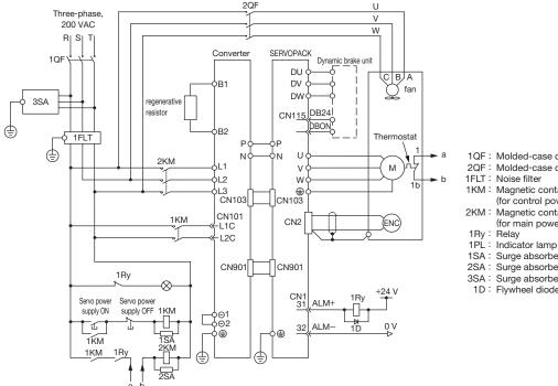
1QF: Molded-case circuit breaker 2QF: Molded-case circuit breaker
